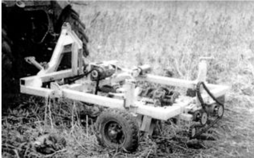
Fig. 2. Overall view of the experimental equipment: the remover with two horizontal cylinders
